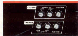
Servo reversing, throw adjustment and sub-trimming can be individually preset on the 2PD control panel.
