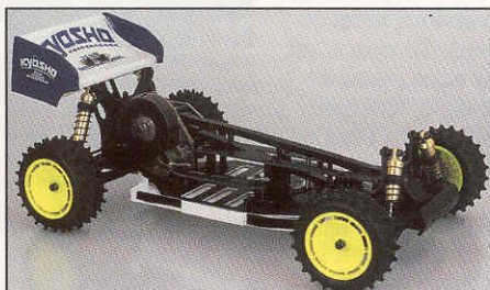
Graphite top and bottom chassis plates offer high strength with low weight. The Lazer ZX layout means quick maintenance.
